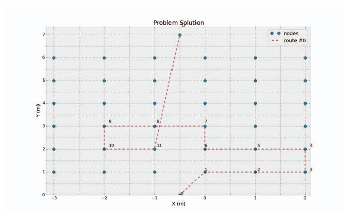
Fig. 4. Open vehicle routing problem solution for a 6x6 grid and energy budget of 30 units. The utility gathered was 14.28.
