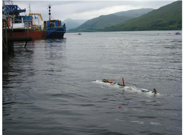
Fig. 1. Nessie AUV during an inspection mission at The Underwater Centre, Fort William, UK. In environment like this the presence of strong tidal currents affect sensibly the energy usage during long-term autonomous missions.
