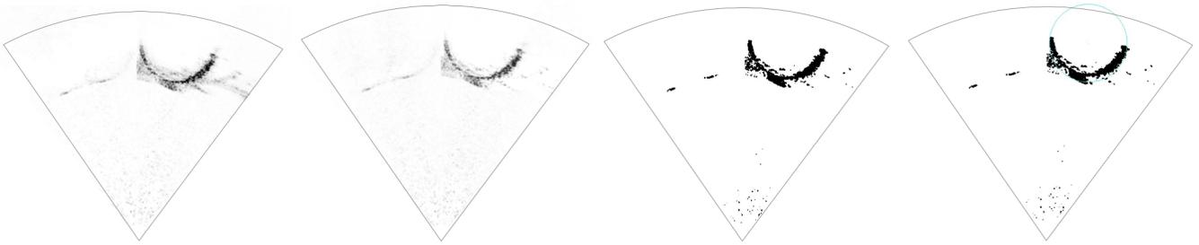
Fig. 4. The various steps in signal processing. From left to right: raw image, average, threshold, hough circle.
