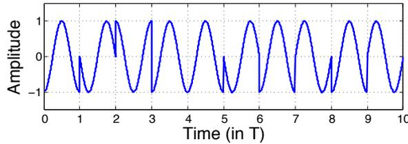
Fig. 2: Example of phased coded radar waveform.
