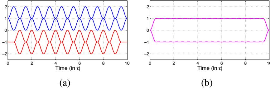
*Fig. 3: (a) envelop of the concatenated micro-chirps (blue curve) and the interlaced concatenated micro-chirps (red curve). (b) full IMCS waveform envelop.*
