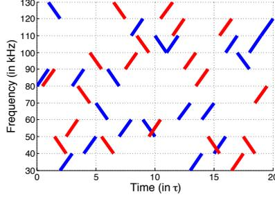
Fig. 4: Example of an IMCS waveform structure in the time-frequency domain. The blue segments represent the micro-chirps of the first series, the red ones represent the second series.
