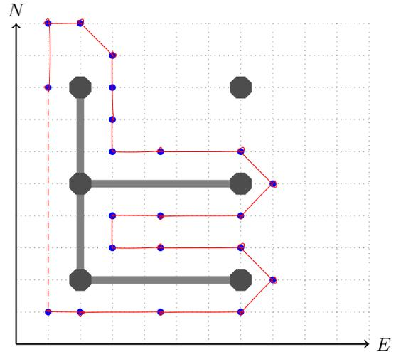
Figure 4. Nessie AUV trajectory plan in north-east plane for an inspection mission around human-made structures. The blue dots represent the trajectory's waypoints while the red line represents the real navigation path. The inspected structure, made of concrete pillars and crossbeams, is represented in grey.
