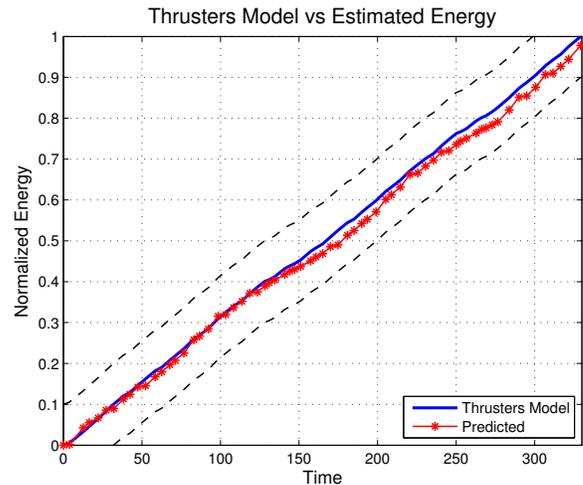
Figure 5. Comparison between thruster's model and predicted energy using the proposed model for inspection mission. The energy values have been normalized to the total resource usage for the final navigation trajectory.
