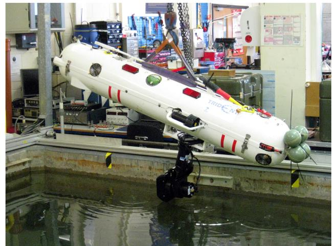
Figure 1. Nessie VII AUV during pre-trial testing inside OSL facilities. The pan-and-tilt unit with sonar has been fitted underneath the vehicle to provide enhanced capabilities for inspection and surveying tasks.
