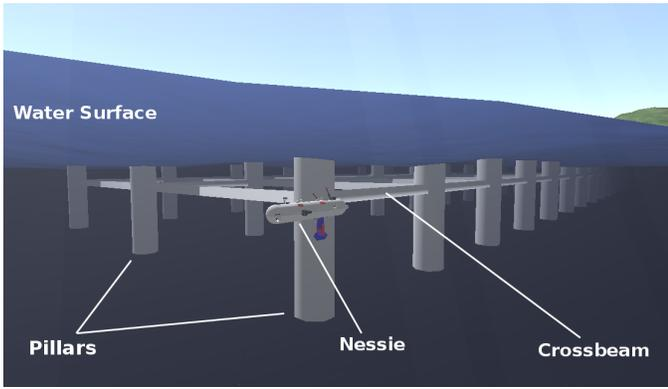
Figure 3. Underwater view of the simulated mission's scenario. The structure to inspect is made by concrete pillars and crossbeams. Nessie VII AUV is collecting data from its sensors while navigating around pillars.
