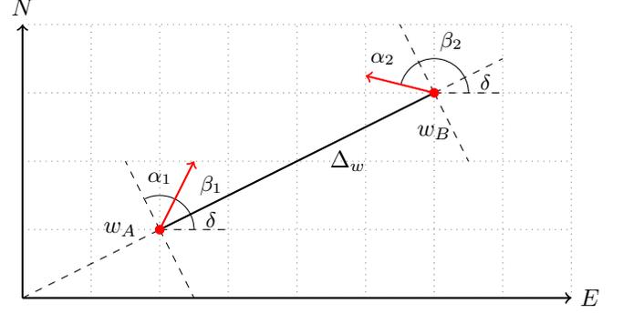
Figure 2. Geometric representation of two waypoints ( $w_A, w_B$ ) with required yaw attitude in north-east plane. The angles  $\alpha$  and  $\beta$  represent the orientation changes needed respectively for *forward* and *lateral* navigation modes while  $\delta$  is the line-of-sight angle between waypoints.
