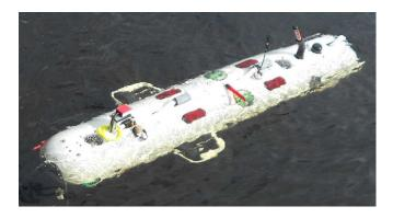
Fig. 5. Nessie is the main research platform of the Oceans System Lab. It is a hover capable torpedo shaped AUV with a variety of sensors that are used for navigation (DVL,Gyro,Compass) as well as a Blueview forward looking sonar for perception.
